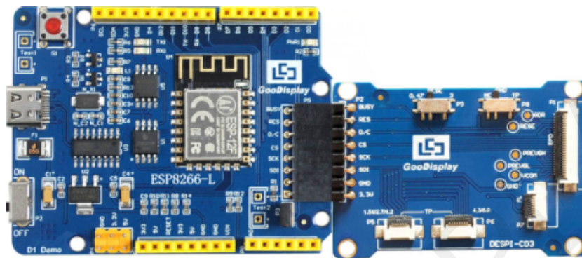
Figure 3 : Connection between ESP8266-L for EPD and DESPI-C03
